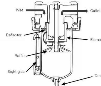
Inspections and maintenance should be carried out regularly after the commissioning. If condensate collects, drain the condensate at brief intervals through the condensate drain plug. The maintenance intervals depend on the operating mode of the filter but should be performed at the latest every 6 months.
